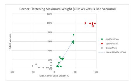
The convex warped sheets (left from the 0 load line) are no problem on the vacuum bed.
